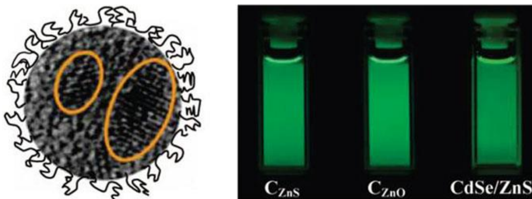
Figure 2.8 CDs doped with ZnS. ( Left ) – Image of ZnS lattice planes within CDs (circled) under HRTEM. ( Right ) – Fluorescence in present in all solutions of CDs/semiconductor composites under UV irradiation.
